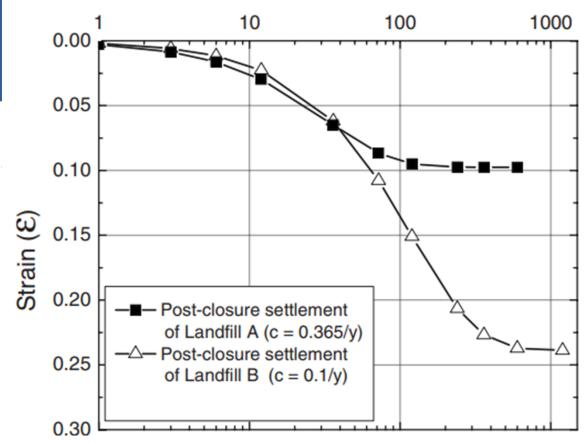
The amount of secondary settlement that has occurred is a function of a compression index and time.
